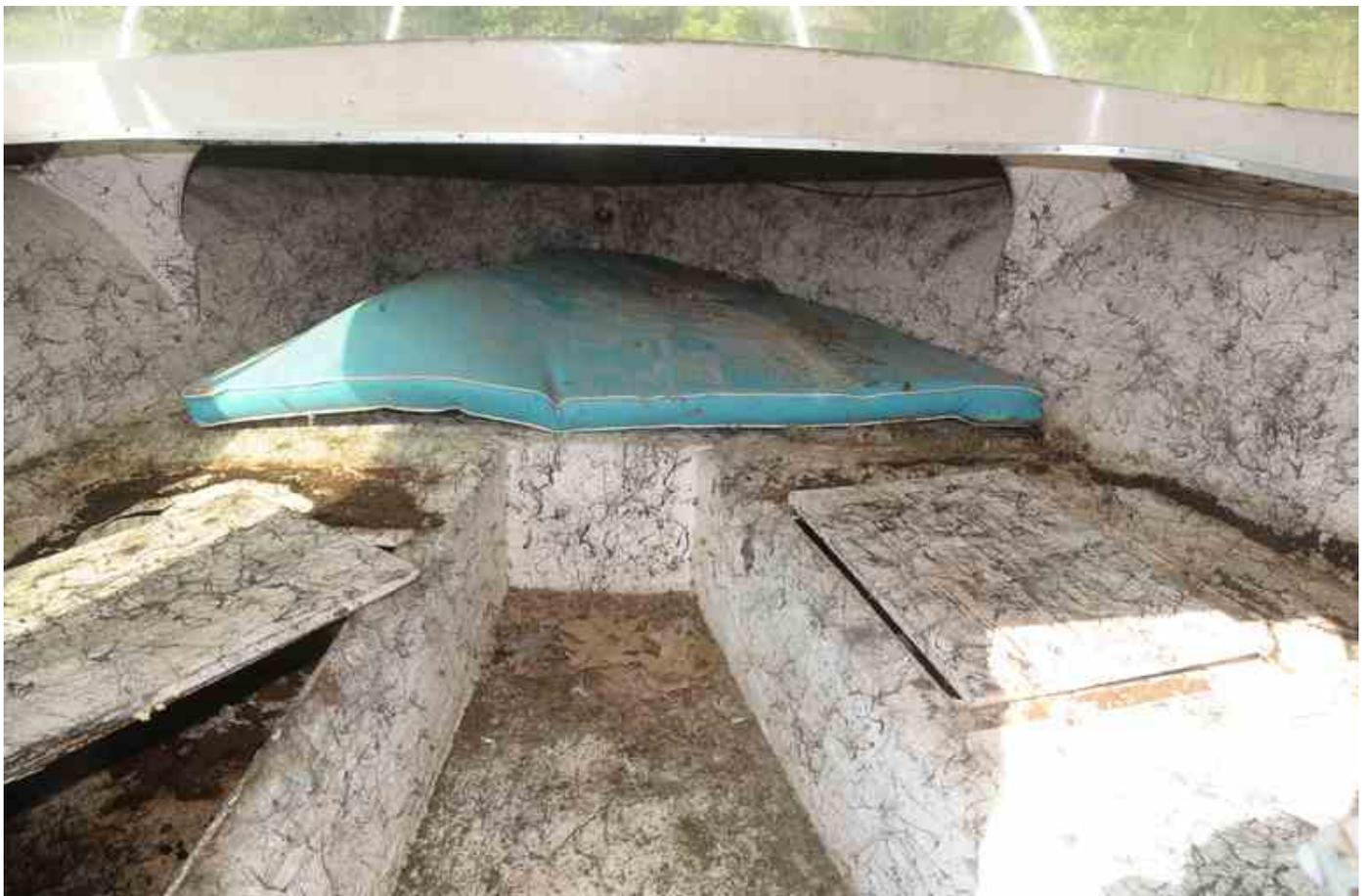
**What I have done so far is taken out all the 500 pounds of waterlogged crap inside it. The sole, bulkhead, and stringers have all been removed, as the exterior of the transom. The transom is about 2” thick, and was an ant farm.**
