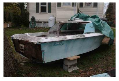
The boat is sitting on wood all along the keel, supported on the sides by blocks- more on that later. Reference the sole and stringer removal. --- Interior before sole removal. Settees cut out.
