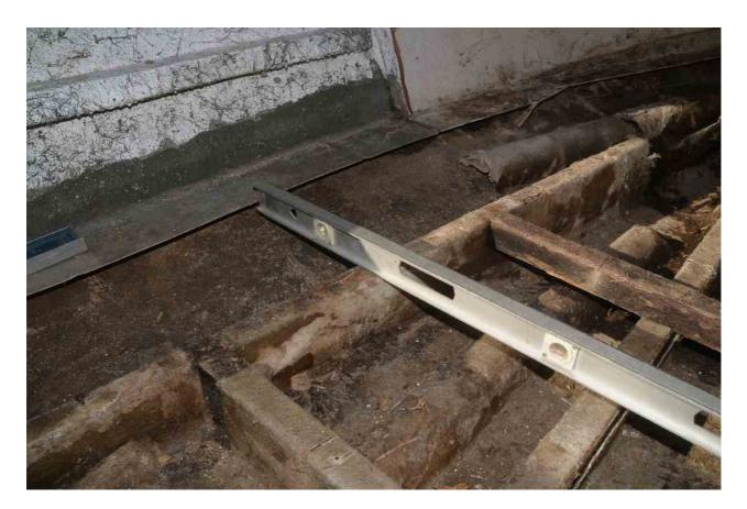
The above shows the port side just aft of the cabin bulkhead. You can see the central stringer starting downward under the floor behind the level. It looks like the sole was supported by just the outside stringers and I'd like to bring that support up for the whole sole, probably by putting a spacer in there.
