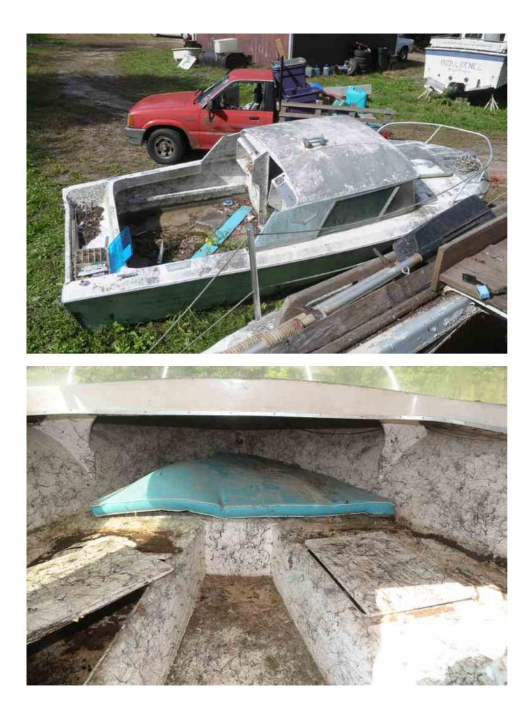
What I have done so far is taken out all the 500 pounds of waterlogged crap inside it. The sole, bulkhead, and stringers have all been removed, as the exterior of the transom. The transom is about 2" thick, and was an ant farm.
