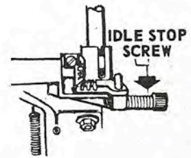
Fig. J43—On all series RD motors before 1960, idle speed is adjusted by the stop screw shown. Screw is located on port side of motor.
