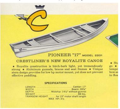
Above: excerpt from the 1961 Crestliner catalog shown on page 1 of this newsletter. Royalite was a laminate of layers of plastic and rubber. Beginning in early 1961 the Pioneer canoe hulls were made by a subcontractor in Rhode Island and the finish work done in the Thompsonville factory.
