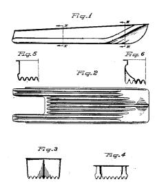
Figure 1 is a side elevation of a boat hull or similar article showing my new design;
